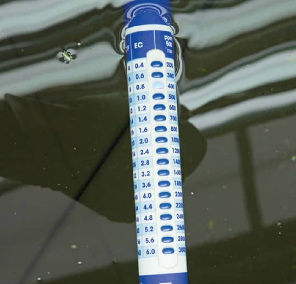
Measure the starting EC after adding water to the reservoir.
